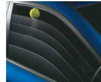
Auto Up/Down Power Window with Pinch Guard
